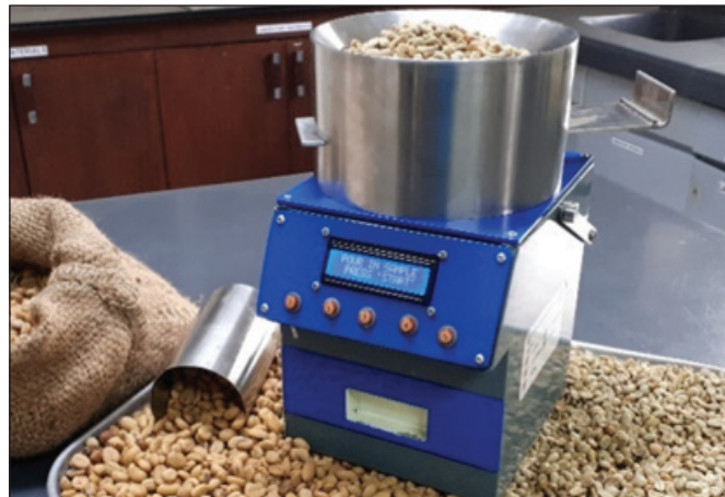
Figure 3. The developed non-destructive coffee moisture meter.
