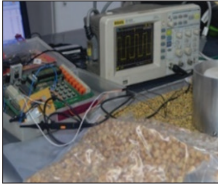
Figure 2. Calibration tests conducted for green coffee beans and coffee parchments for the prototype unit test chamber of the non-destructive coffee moisture meter
