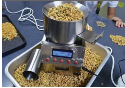
Figure 2. Calibration tests conducted for green coffee beans and coffee parchments for the prototype unit test chamber of the non-destructive coffee moisture meter
